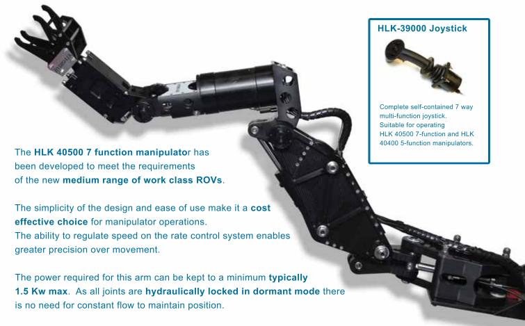
The arm can be mounted on either side of the ROV by virtue of a unique slew bracket which can be installed for **starboard or port mounting**. This enables an upper arm range which can work from below the ROV to points close to the standard badge bar. Jaws with an opening range of 0 - 152mm are included as standard.
