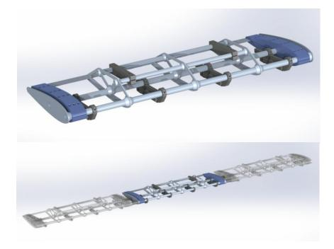
The floatation panels can be inserted, increased or removed one by one to adapt to overall ROV setup. As the frames are combinable – either fixed or even with hinges to keep the low
