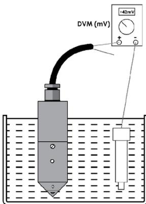
Plastic container filled with 3% Salinity artificial seawater solution.
