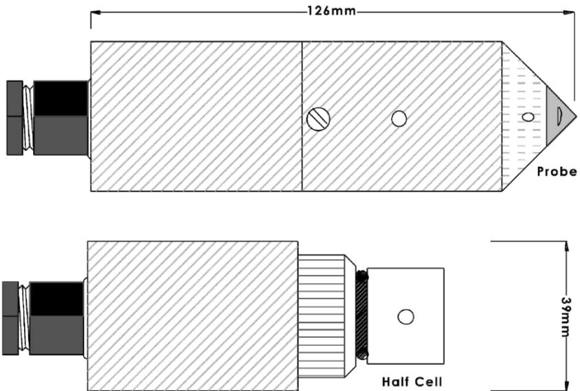
Fig.1 - UCP 1A Contact Probe
