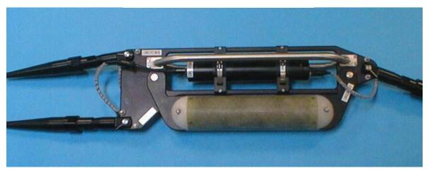
Figure 8. Telemetry tow bar with interconnect and tow cables attached.
