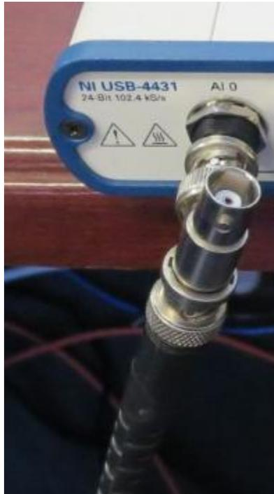
This photo shows the BNC F-M-F Tee connector plugged into the AI 0 (trigger input) channel, with the 12" RG-58 BNC patch cable connected to one female end
