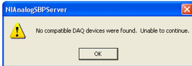
If either of these messages occurs, just plug the USB connector into the CTI 5-BNC box and try again.
